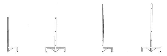
These support frames are available in depths of 300, 400 and 500 mm and are assembled in modules 800 mm in width.
